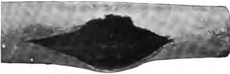
FIG. 22a.—Ruptured Blow-off Pipe.
